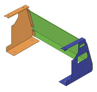
Set the top panel into place and add the washers and Spin knobs.
