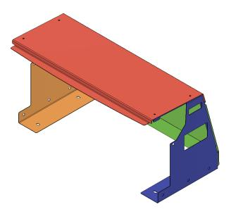
There are 2 brackets that attach to the side walls either the small 1/4-20 screws. The top of the brackets line up under the top of the side walls and match the slotted holes for the top. You can add these or not. They add a little extra structure.
