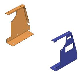
Lift the Center wall panel in and into place with the PEM Studs into each hole and slot. Add the large washers and Spin knobs. Keep a little loose till end.
