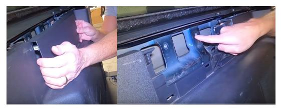
Place a rag or piece of cardboard in the gap between the body tub and the inner plastic to avoid dropping a bolt between them.
