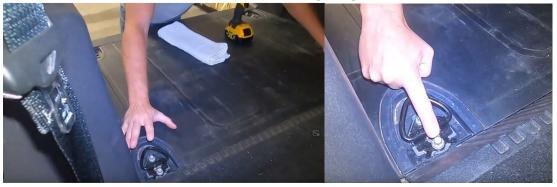
Remove the plastic side panels covering the factory bolt locations on the body tub (used for main bracket hardware)
