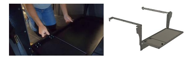
Raise the wall to the vertical position and ensure there is enough gap between the metal parts. If you need to increase the gap insert the cardboard shim and slowly adjust the vertical frames outward to ensure proper gap. Insert the quick release pins in the top of the wall. (1:02:30) Tighten all vertical frame and lower wall bolts to ensure the wall retains the gaps (1:03:50)
