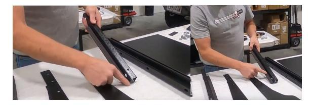
Attach the vertical frames with the flat flange facing outward with the gap at the bottom to the Wing Walls.
