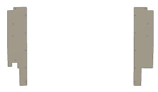
Identify Driver and Passenger wingskins, (Driver has cutout for wiring harness) (33:30) Place the wingskin on top of the side frames placing them just under the body tub and matching the holes in the side frames. Place the tie down rails on top of the wing skin with the flange inward and secure with carriage bolts. (35:30) place washers and nuts on all carriage bolts about ½ way. Align the frame system parallel to the wall to ensure a good 90 degrees and tighten all nuts to ¾.
